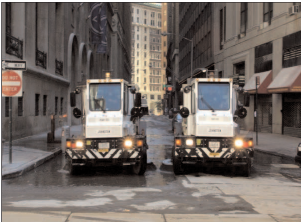
Mechanical Broom Cleaning Operation
